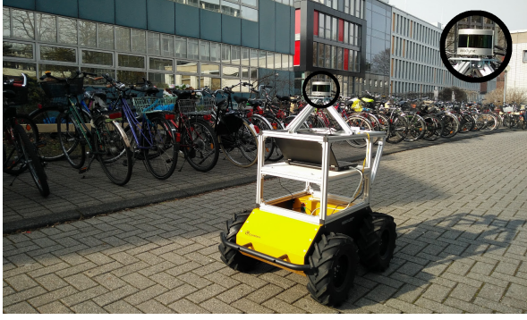
Fig. 3. Robot equipped with a 16-beam Velodyne used for our experiments.
