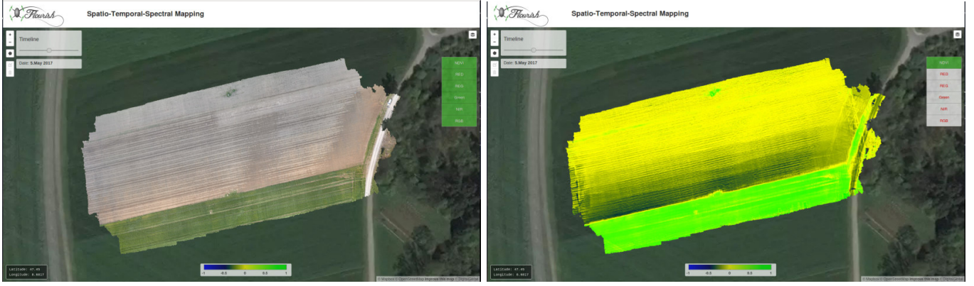
Fig. 9. Visualization interface for the spatio-temporal-spectral database showing both RGB orthomosaics (left) and corresponding index maps (right) for a sugar beet field over time. The user can select spectral layers to view a georeferenced reflectance orthomosaic corresponding to a wavelength band, view the color orthomosaic, and toggle through all available surveys using the timeline.
