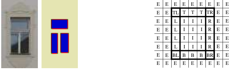
Figure 1: Labeled image. Image and the labeled image encoded in color (left) and allowed configuration of labels (right), E - external label (represents a facade), I - internal windowpane label, L,R,T,B are left, right, top, bottom edge respectively and TL, TR, BL, BR are corners.
